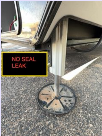
Comparison of actuator that is good with NO seal leak
