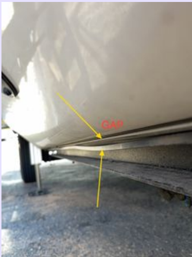
Underbelly Light bar glue failing
