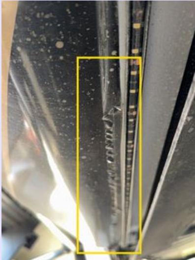
Underbelly decals peeling away
